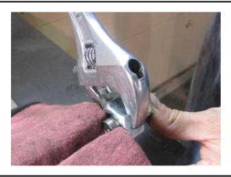
7. Release the valve from the vise and remove the spring to insert the supplied *hardened steel shims* into the valve.
