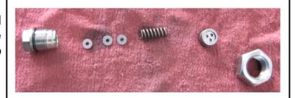
8. Re-insert the spring and cap ensuring not to lose the small pin in that is inside the valve cap.
