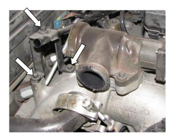
13. Reinstall the clamps back onto the EGR pipe and Re tilt the pipe back into position. Tighten one side slightly to allow enough movement to connect the other side, torque to 89 in/lbs once both sides are correctly aligned.
