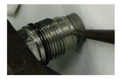
10. Reinstall fuel pressure relief valve back into the fuel rail. (torque to 76 ft/lbs)
