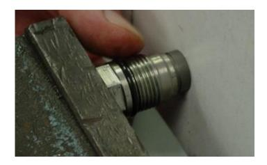
9. Using a punch and small hammer re-strike the factory indentations along the lip where the valve casing covers the valve cap (3 places). You may need to rotate the valve to access the three locations by slightly loosening the vise ensuring the cap stays fully seated in the valve while it is being rotated.
