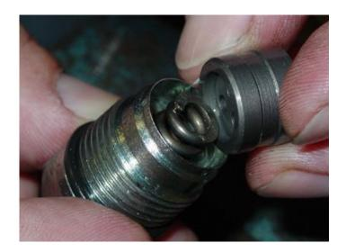
8. Place the valve back into the vise with a piece of cardboard behind the valve cap to prevent damage to the valve seal surface. Tighten the vise until snug so the valve cap re-enters the valve until fully seated.
