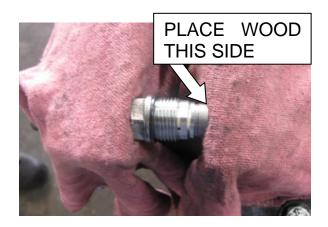
10. Using a small hammer and punch re-strike the factory indentations along the lip where the valve casing covers the cap (3 places).
