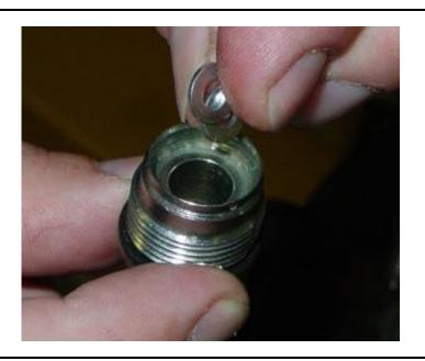
7. Reinsert the valve spring then the cap.
