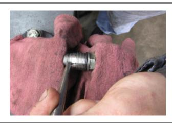
11. Reinstall the fuel valve and torque to 76 ft/lbs.
