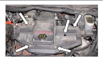
Loosen/remove the two clamps that hold the EGR tube that crosses the front of the engine, and tilt the tube out of the way.
