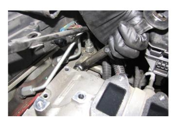
12. Reinstall the air horn insuring to align the gasket holes and reinstall the dipstick tube to the air horn. (Torque to 18 ft/lbs)
