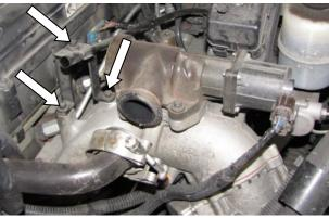
Remove the fuel rail valve located at the front of the fuel rail. (18mm wrench)
