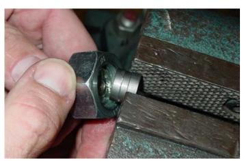
6. Remove the spring and insert the supplied *hardened steel shims* into the valve.
