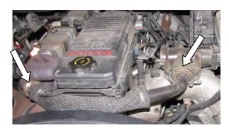
3. Remove the bolt that holds the dipstick tube to the air intake horn bracket then remove the six bolts that hold the air intake horn to the manifold (10mm socket and wrench) gently slide the intake horn forward to access the front of the fuel rail.
